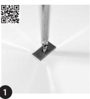
Fix mounting plates with screws provided (min. 2 per 500mm/20").
